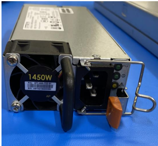
Figure 26. 1450 W power supply
