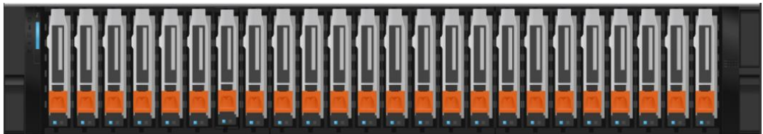
Figure 27. 24-drive 2.5-inch 2U NVMe expansion enclosure (front)
