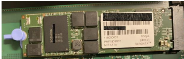
Figure 20. Internal M.2 boot module
