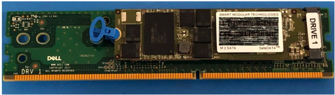
Figure 4. Internal M.2 boot module
