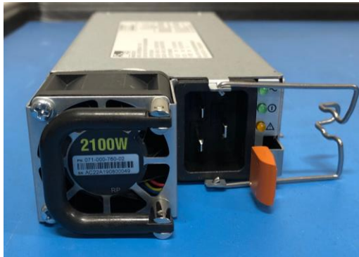
Figure 10. 2100 W power supply
