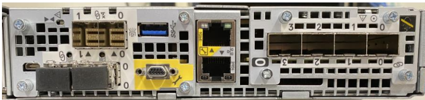
Figure 24. Embedded module with 4-port card
