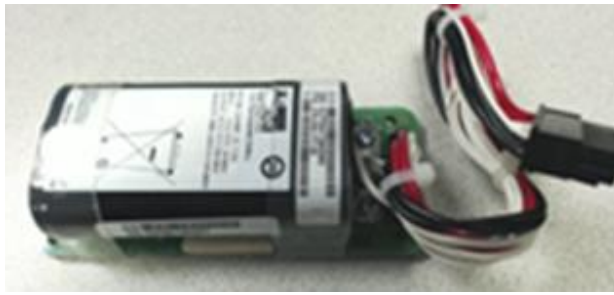
Figure 6. Battery backup unit
