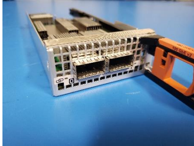
Figure 31. 100 GbE optical I/O module
